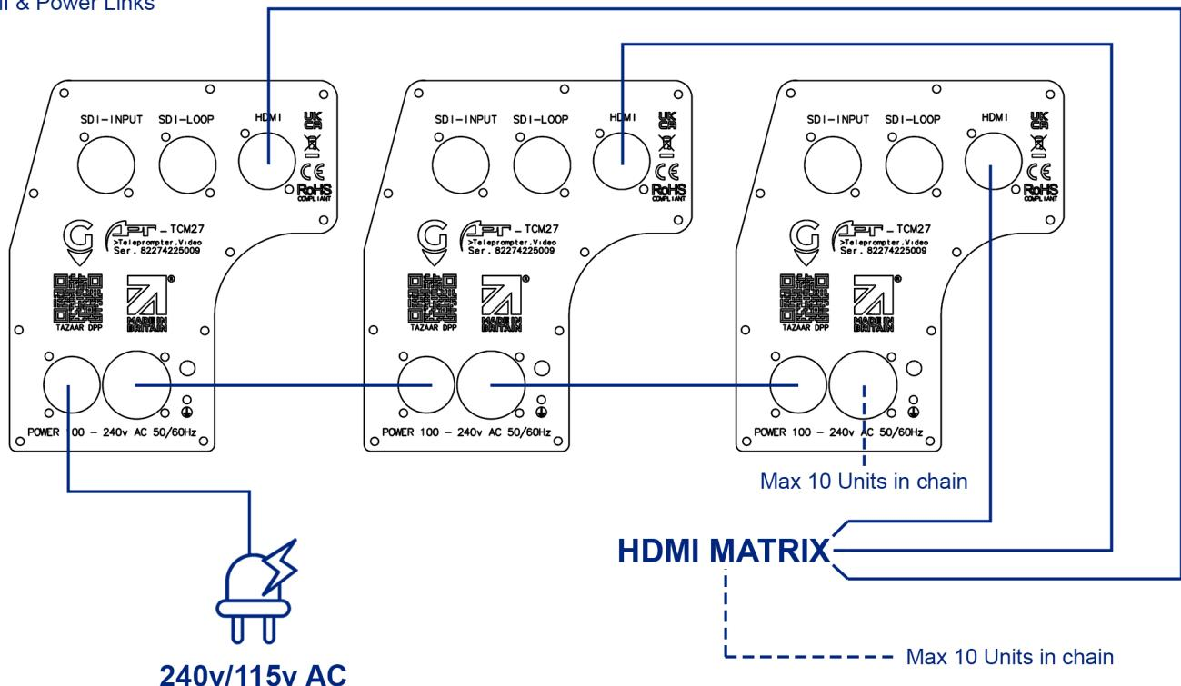
Please note only one input connection configuration can be used at a time
